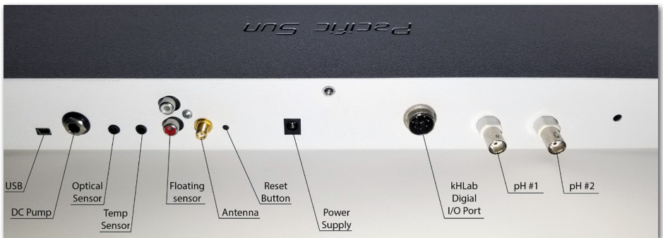
Kore 7th Dosing Station back panel
